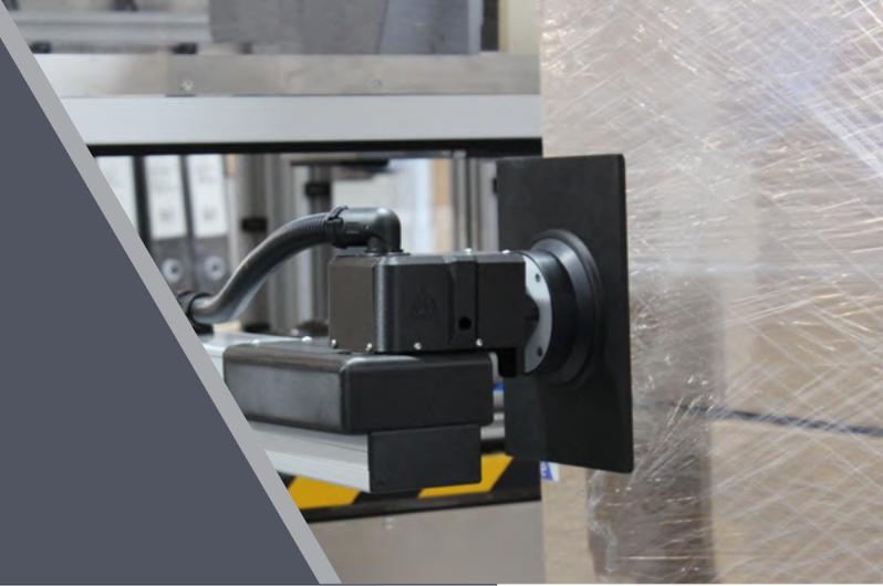
Introducing the Vector, a low maintenance high performance tertiary pallet labeller, capable of printing up to four labels on three sides with two pallet stop positions.
